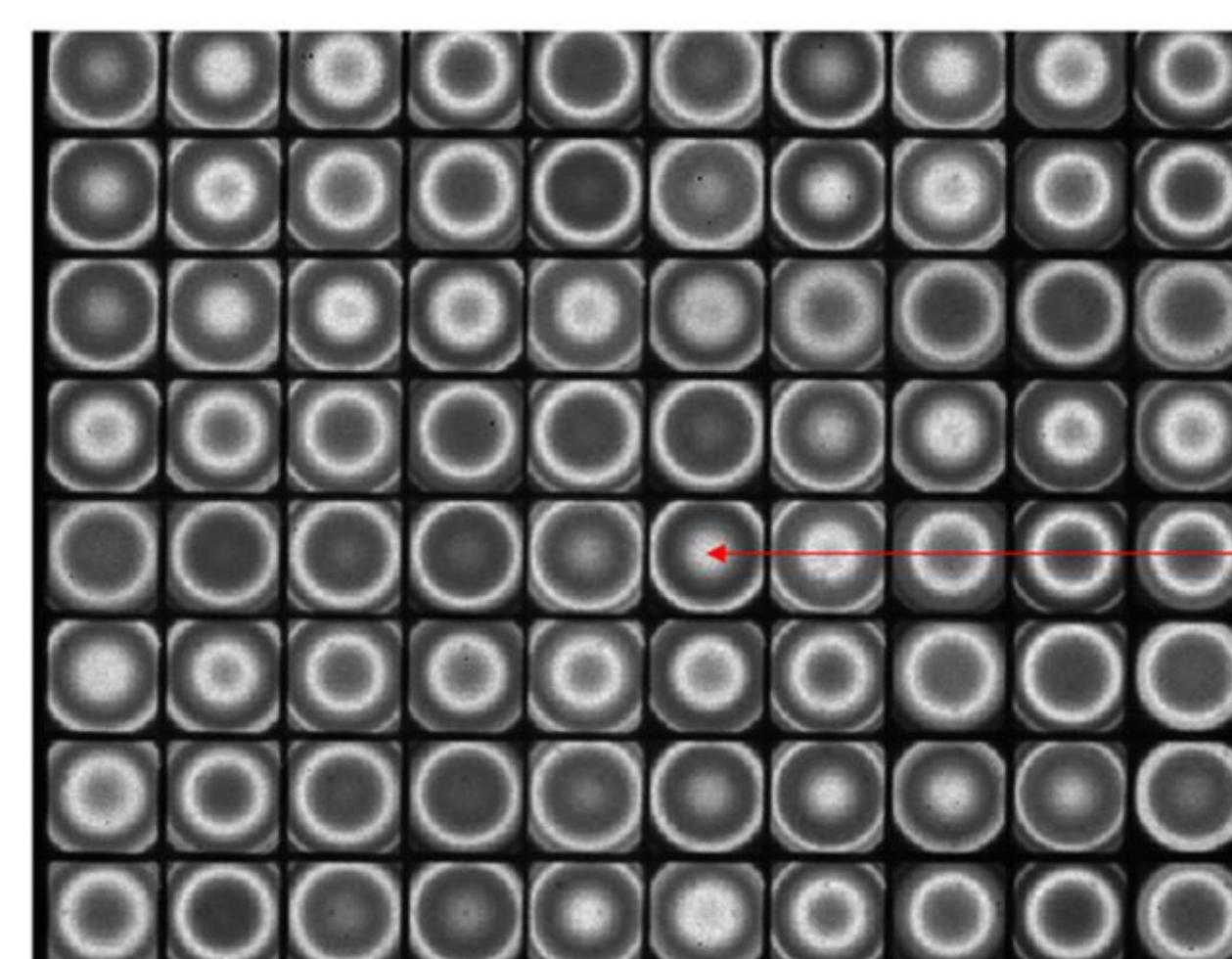
Frame acquisition at 1607 nm under uniform and monochromatic illumination, showing Fabry-Perot ring pattern collection corresponding each one to one interferometer at a given thickness
